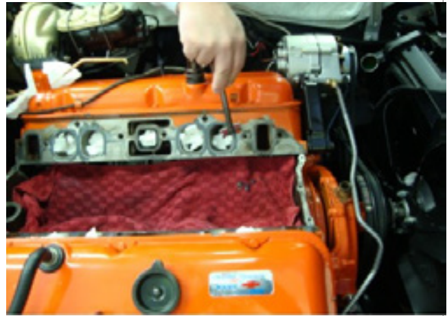
New gaskets installed
