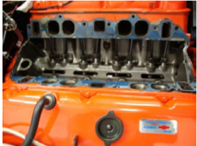
Old gaskets to be removed
