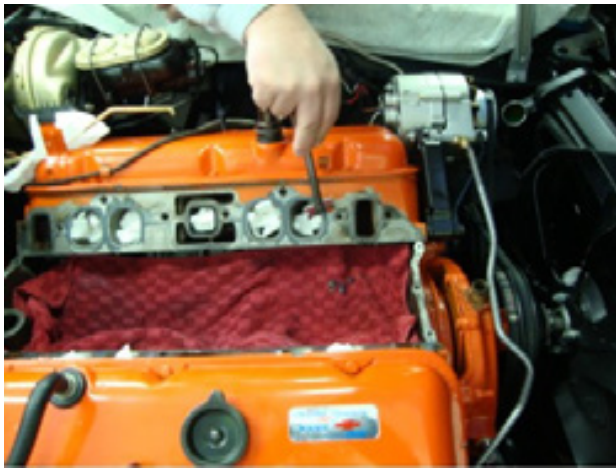
Cleaning of old gaskets
